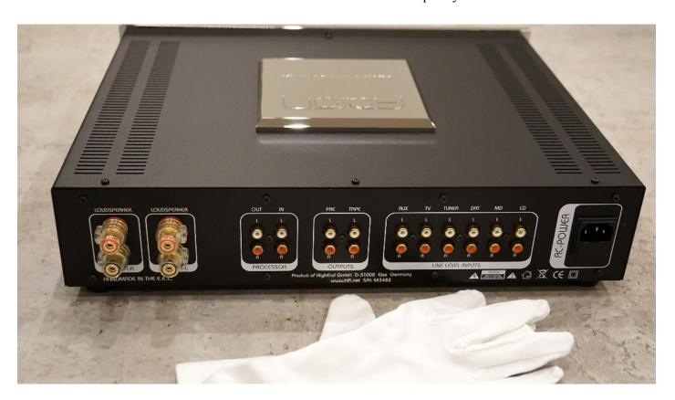
That aside, it's measurements are 440mm wide X 108mm high X 375mm deep and chassis/cover is made from plate steel with a flecked black finish. Weight is 15.5kg.
